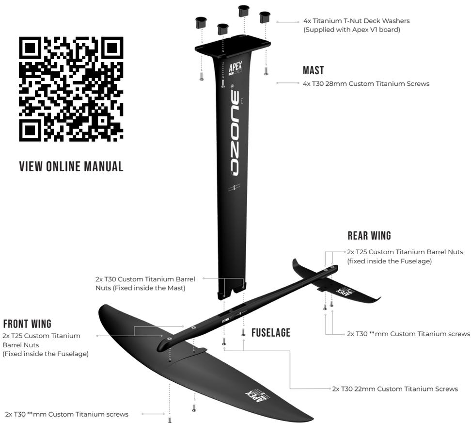
*\*\*Refer to the screw pocket inside the wing cover OR online manual for screw length)*
